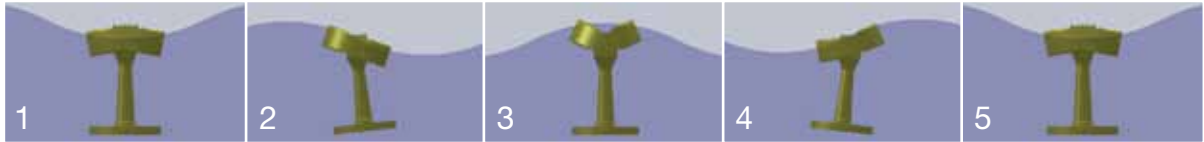
COLUMBIA POWER's wave power system: The wings and vertical spar react to the shape of the passing ocean swell. Each wing is coupled by a drive shaft to turn its own rotary generator.
