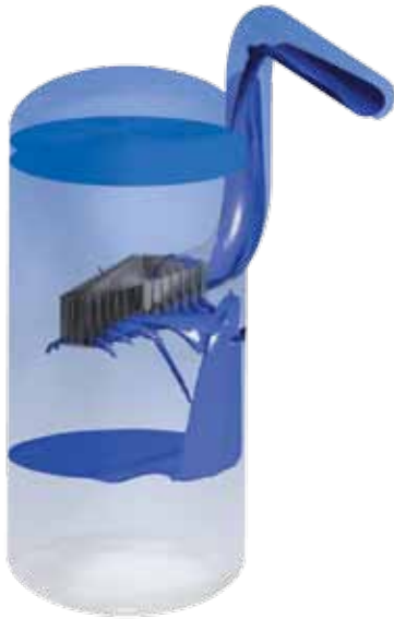
Analysis of a vertical production separator with a vane-type inlet device shows that the inlet pipe keeps much of the liquid on one side of the vessel — leading to non-optimal separation.
