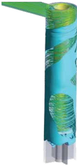
Simulation of a vertical cyclone vessel designed to remove bulk liquid from the feed stream. Pathlines of primary gas phase show where the liquid has a concentration of more than 25 percent.
