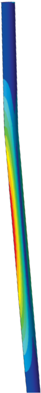
Nonlinear springs were used to represent soil forces acting on the conductor.
