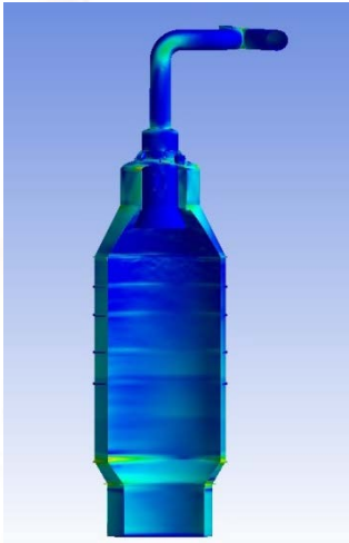
Fitness for Service Assessment of API 620 Blow Tanks, Design of New 2205 Duplex Shell & Vibration Measurements & Analysis (80 ft H)
